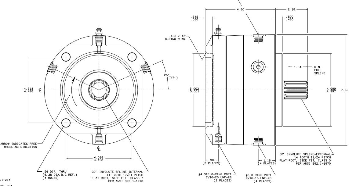
IF USED IN SUMP CONDITION REPLACE THIS O-RING PLUG WITH A VENTED TYPE PLUG.
