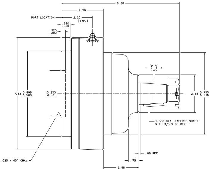
LOAD CAPACITY @ 100 RPM AND B10 = 6,500 HRS 325 RPM AND B10 = 2,000 HRS
