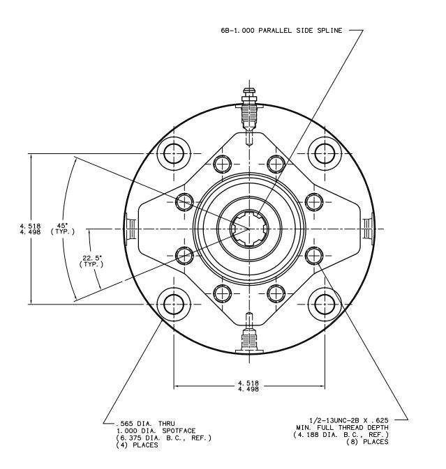
ECO S-1686 5. 03 **-** 2. 18 **-** 1. 58 -(2) PLACES . 295 . 280 <del>---</del> 1.38 --FULL SPLINE 4. 999 4. 997 7.63 DIA. MAX. .065/.055 x 45° CHAM. #6 SAE 0-RING PORT -9/16-18UNF-2B (2) PLACES - 1. 13 -(2) PLACES 30° INVOLUTE SPLINE-EXTERNAL 14 TOOTH 12/24 PITCH FLAT ROOT, SIDE FIT, CLASS 5 PER ANSI B92. 1-1970 #4 SAE O-RING PORT 7/16-20UNF-2B (2) PLACES
