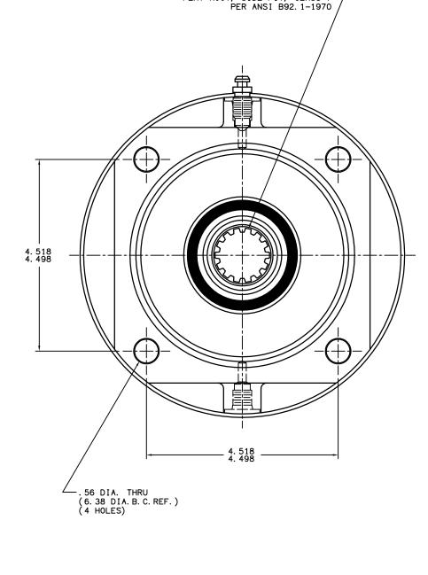
30° INVOLUTE SPLINE-INTERNAL — 14 TOOTH 12/24 PITCH FLAT ROOT, SIDE FIT, CLASS 7
